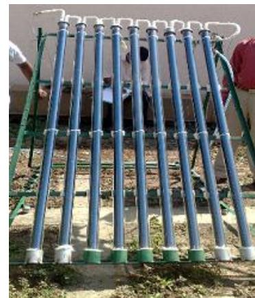
Fig.1. Frontal view of nine tubes evacuated collector.
